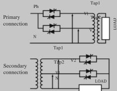
The operating region of control will determine the number of taps required but a maximum of 4 is usually sufficient.
