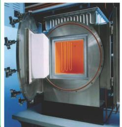
Our client successfully tested a feature of the EPower controller in a new way alongside their world leading brand of (MoSi2) heaters known as Kanthal Super. A key feature of MoSi2 heaters is the relationship between impedance and heater temperature.
